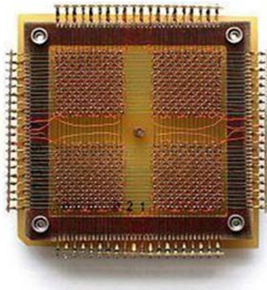
Figure 1.6: A 32 x 32 core memory plane storing 1024 bits of data.
