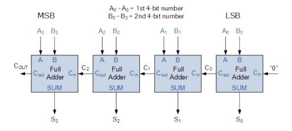
The output carry from one full-adder connected to the input carry of the next full-adder.
