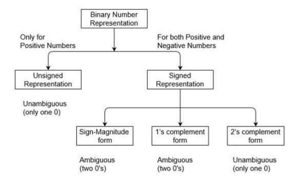
There are three types of representations for signed binary numbers. Because of extra signed bit, binary number zero has two representation, either positive (0) or negative (1) These are:
