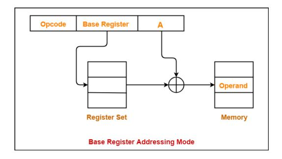
The difference between the two modes is, an index register is assumed to hold an index number that is relative to the address part of the instruction. A base register is assumed to hold a base address and the address field of the instruction gives a displacement relative to this base address.
