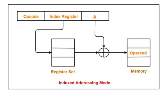
The index register is a special CPU register that contains an index value.
