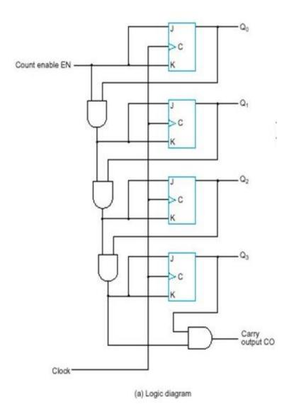
J and K inputs of flip-flops are driven from separate AND gates which are also supplied with signals from the input and output of the previous stage. These additional AND gates generate the required logic for the JK inputs of the next stage.
