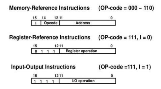
The operation code (opcode) part of the instruction contains three bits and the meaning of the remaining 13 bits depends on the operation code encountered.
