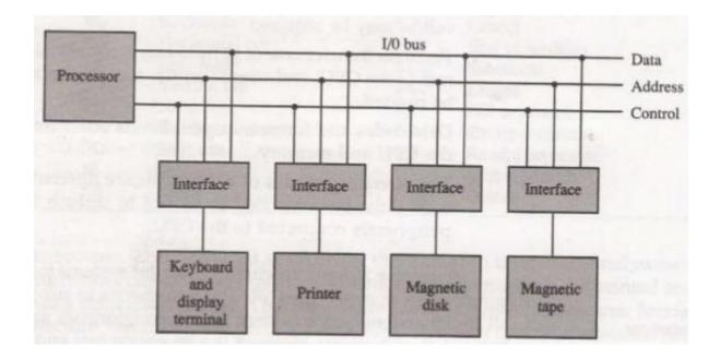
The I/O bus consists of data lines, address lines, and control lines. The magnetic disk, printer, and terminal are employed in practically any general-purpose computer. The magnetic tape is used in some computers for backup storage. Each peripheral device has associated with it an interface unit.
