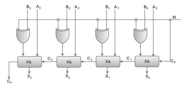
The mode input M controls the operation. When M = 0 the circuit is an adder and when M = 1 the circuit becomes a subtractor.
