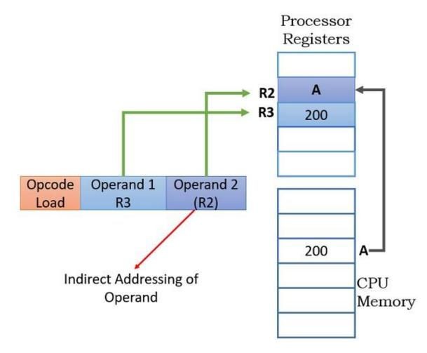
Before using a register indirect mode instruction, the programmer must ensure that the memory address of the operand is placed in the processor register with a previous instruction.
