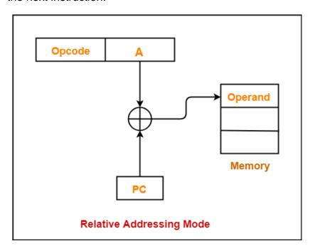
To clarify **with an example**, assume that the program counter contains the number 825 and the address part of the instruction contains the number 24. The instruction at location 825 is read from memory during the fetch phase and the program counter is then incremented by one to 826 + 24 = 850. This is 24 memory locations forward from the address of the next instruction.
