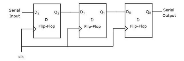
The output of a given flip-flop is connected to the D input of the flip-flop at its right. The clock is common to all flip-flops.
