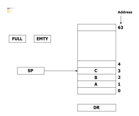
Three items are placed in the stack: A, B, and C, in that order. Item C is on top of the stack so that the content of SP is now 3.
