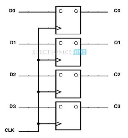
The common clock input triggers all flip-flops on the rising edge of each pulse, and the binary data available at the four inputs are transferred into 4-bit register.
