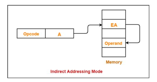
Control fetches the instruction from memory and uses its address part to access memory again to read the effective address.
