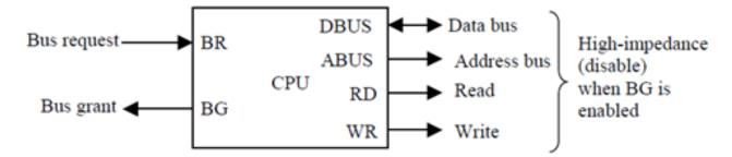
relinquish control of the buses. When this input is active, the CPU terminates the execution of the current instruction and places the address bus, the data bus, and the read and write lines into a high-impedance state. behaves like an open circuit, which means that the output is disconnected and does not have a logic significance.
