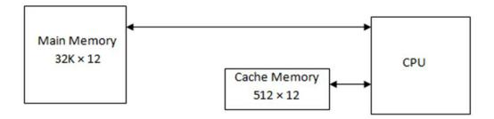
The cache memory access time is less than the access time of main memory The cache is the fastest component in the memory hierarchy The fundamental idea of cache organization is that by keeping the most frequently accessed instructions and data in the fast cache memory.
