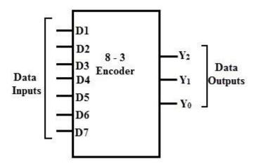
An octal to binary encoder has 8 input lines D0 to D7 and 3 output lines Y0 to Y2.
