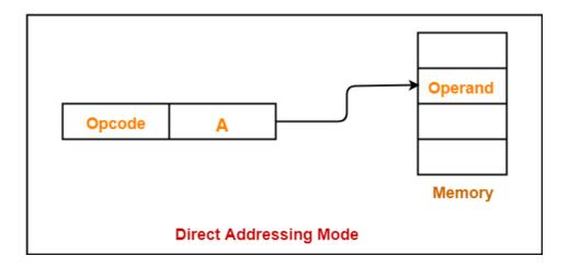
The operand resides in memory and its address is given directly by the address field of the instruction. In a branch-type instruction the address field specifies the actual branch address.
