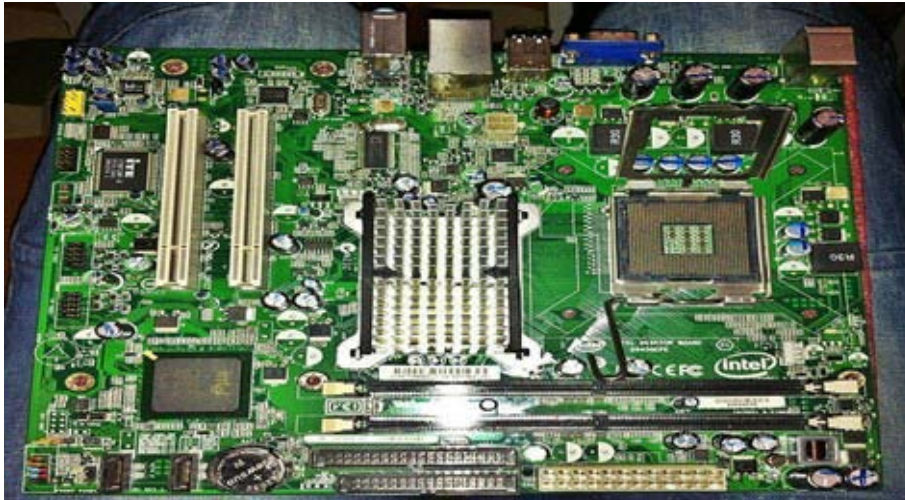
Figure:1.14d: Intel D945GCPE A microATX Motherboard LGA775 for Intel Pentium 4, D, XE, Dual-Core, Core 2 (circa 2007)
