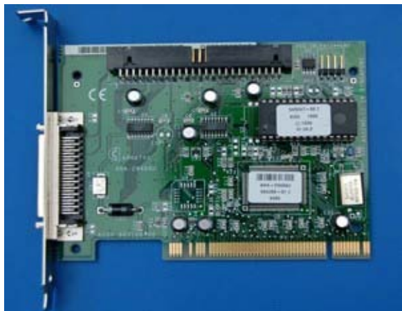
Figure 1.14a: A typical 32-bit, 5 V-only PCI card, in this case, a SCSI adapter from Adaptec.
