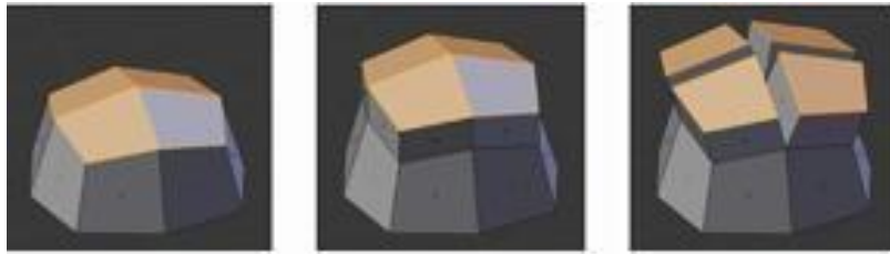
Title-Img 4. 11 Selection of multiple faces, extruded using extrude region and Extruded using Extrude Individual
