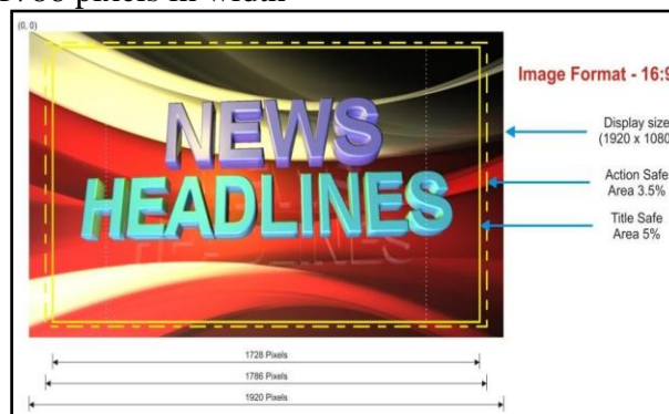
(Fig 08) Action Safe and Title Safe Margins in High Definition (16:9) Display [Created by author]
