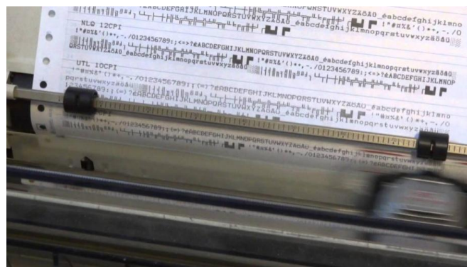
Fig 3.12 Dot Matrix Printing (Picture source: youtube.com)
