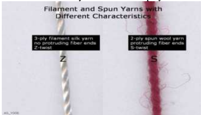
(Figure 8.6 The difference between thread and yarn)
