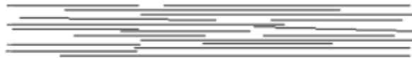
(The structure of para-aramid fiber ) The aramid fiber in Figure 7.16 is composed of fully stretched chains)
