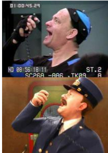
Fig. 1.6: A Movie Star wearing a Motion Capture Suit and the Output
