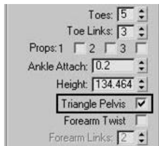
Fig. 2.4: Biped Creation Rollout showing Triangle Pelvis Option
