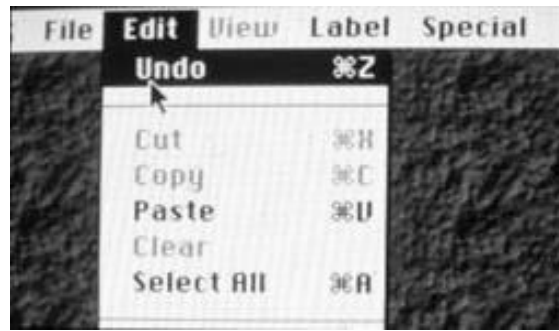
Figure: 1.5 The design minimizes hazards and the adverse consequences of accidental or unintended actions. Courtesy
