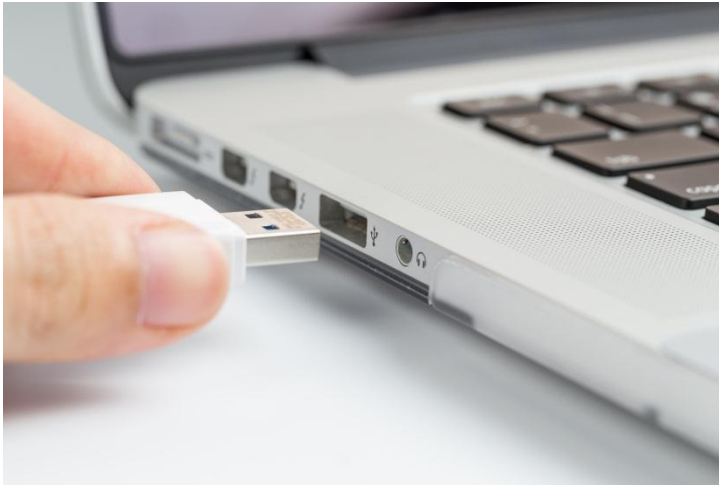
Fig. 2.8: It is an external bus standard that supports data transfer rates of 12 Mbps and is good for supporting up to 127 devices.
