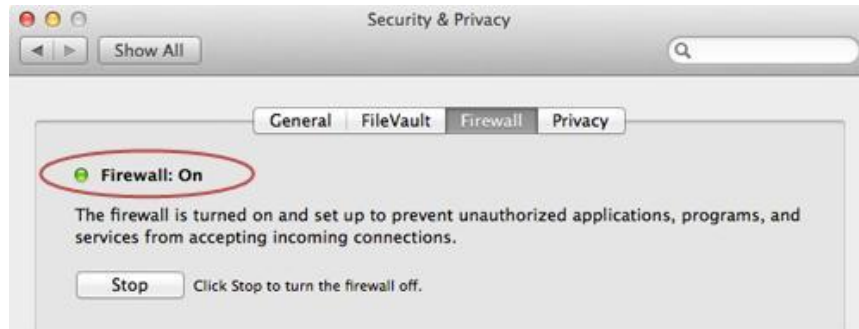
Figure 34: Turning on firewall
