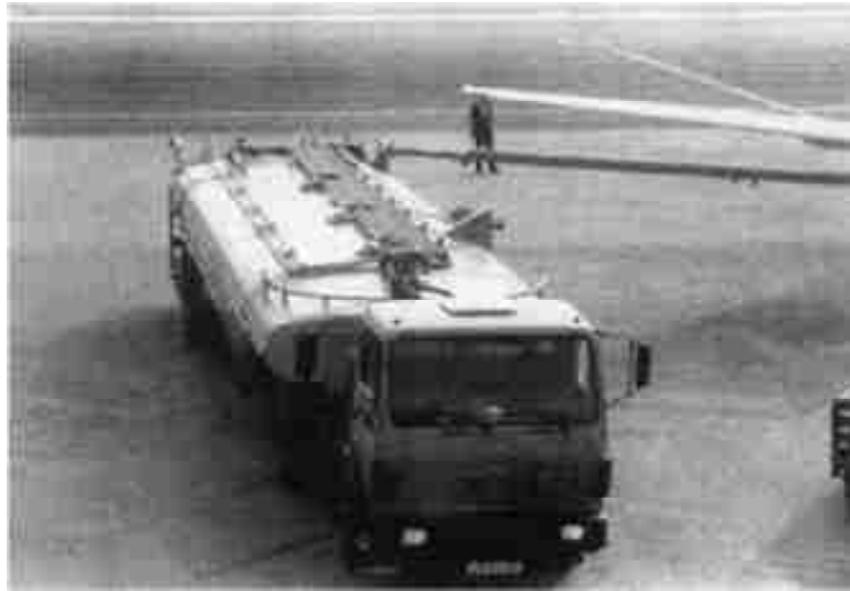
Fuelling from Apron Tanker System
